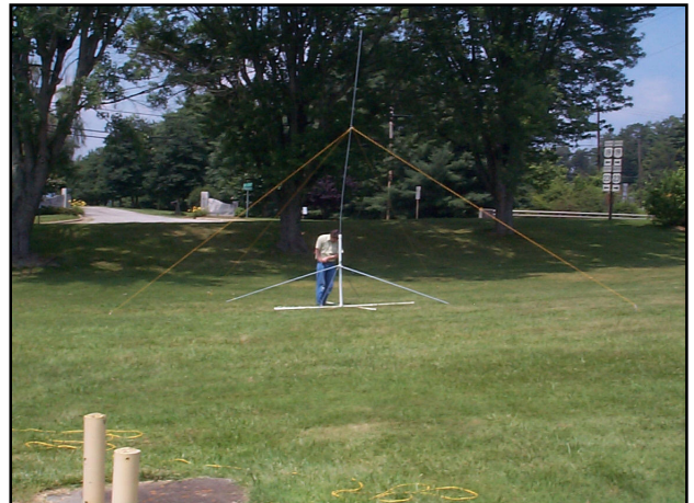
K4AVL assembles his homebuilt 20-meter vertical.
